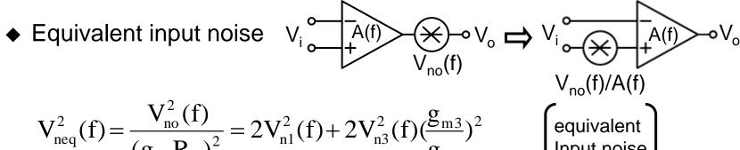
$$V_{\text{neq}}^{2}(f) = \frac{V_{\text{no}}^{2}(f)}{(g_{\text{m1}}R_{\text{o}})^{2}} = 2V_{\text{n1}}^{2}(f) + 2V_{\text{n3}}^{2}(f)(\frac{g_{\text{m3}}}{g_{\text{m1}}})^{2} \qquad \text{equivalent Input noise}$$
