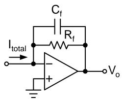
$$V_{o} = -I_{total} \frac{1}{\frac{1}{R_{f}} + SC_{f}} = I_{total} \times \frac{R_{f}}{1 + SR_{f}C_{f}}$$
