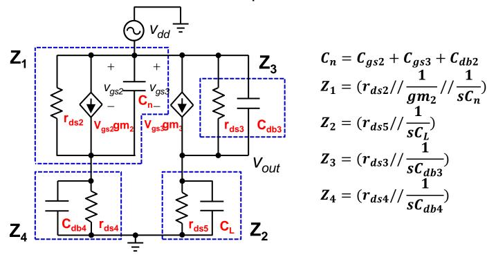
v<sub>out</sub> / v<sub>dd</sub> transfer function derivation
